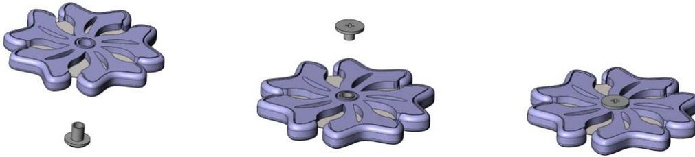
3. Carefully hold this assembly in one hand and insert the screw into the base of the bolt. Use a Phillips screwdriver to tighten the screw. I find that if I place my left thumb on the base of the bolt while turning the screwdriver with my right hand I can keep the bolt from spinning. You only have to turn the screw until it is no longer loose—it will start to spin on your thumb as you turn the screwdriver indicating that it is tight enough.
