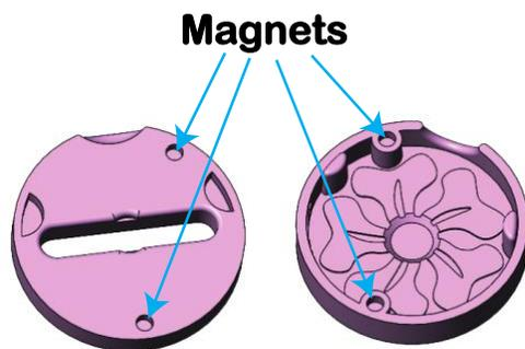
4. Also note that there are thumb holes in the top and bottom of the case. They make it easier to open the case, and they also make it easier to see how to align the case so the magnets and tabs snap into place.
